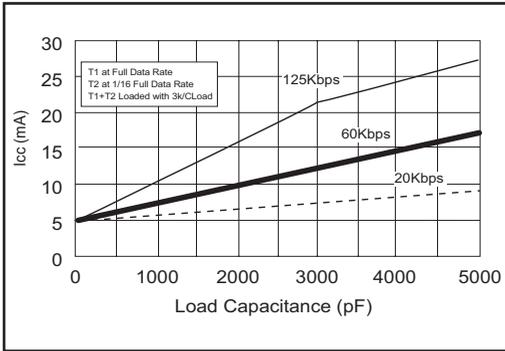
Figure 1.  $I_{cc}$  vs Load Capacitance for the SP3220EB.
