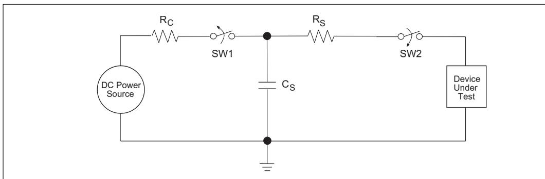
Figure 20. ESD Test Circuit for Human Body Model
