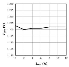
Figure 5: XR76112 Load Regulation, V<sub>IN</sub>=12V
