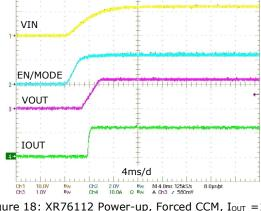
Figure 18: XR76112 Power-up, Forced CCM, I<sub>OUT</sub> =12A
