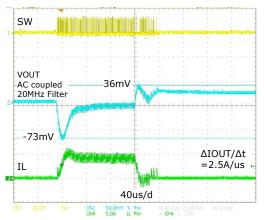
Figure 13: XR76108 Load Step, DCM/CCM, 0A - 4A - 0A
