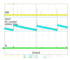
Figure 8: XR76112 Vout Ripple is 22mV at 0A, DCM
