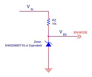
Figure 34: Selecting DCM/CCM by Deriving EN/MODE from V<sub>IN</sub>
