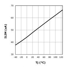
Figure 12:  $I_{\text{LIM}}$  vs. Temperature
