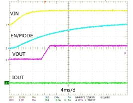
Figure 19: XR76112 Power-up, DCM / CCM,  $I_{OUT} = 0A$
