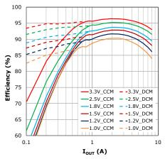
Figure 23: XR76108,  $5V_{IN}$ , 600kHz,  $1\mu H$
