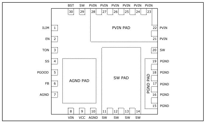
Figure 4: XR76108 / XR76112 Pin Assignment
