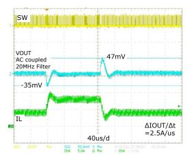
Figure 14: XR76108 Load Step, Forced CCM, 4A - 8 - 4A
