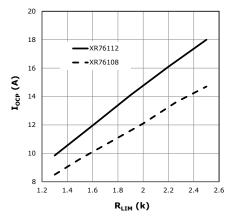
Figure 22: Typical I<sub>OCP</sub> versus R<sub>LIM</sub>
