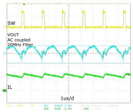
Figure 7: XR76112 V<sub>OUT</sub> Ripple is 14mV at 12A
