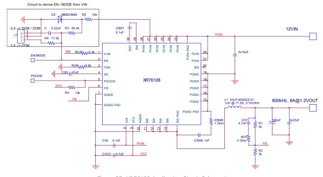
Figure 37: XR76108 Application Circuit Schematic
