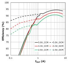
Figure 27: XR76108, 22V<sub>IN</sub>, 400kHz, 3.3µH
