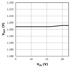
Figure 6: XR76112 Line Regulation, I<sub>OUT</sub>=12A
