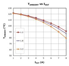
Figure 30: XR76108 Package Thermal Derating, 5VIN
