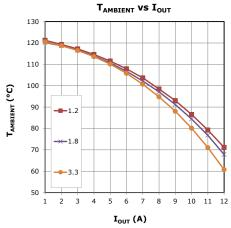
Figure 32: XR76112 Package Thermal Derating,  $5V_{\text{IN}}$
