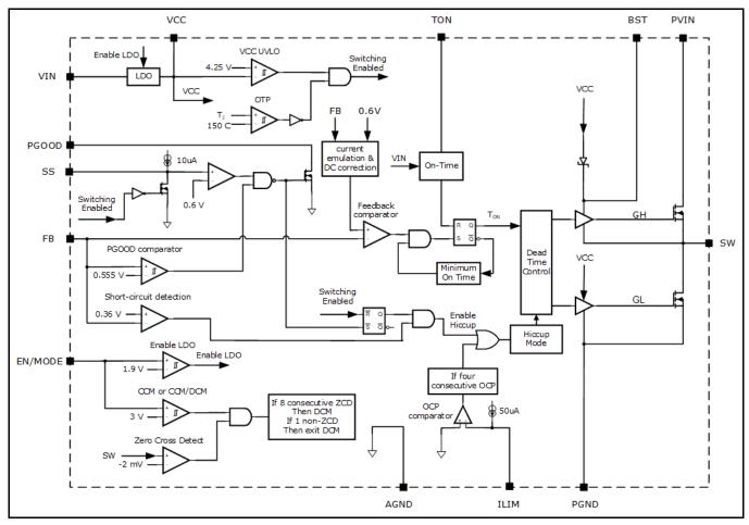
Figure 3: XR76108 / XR76112 Block Diagram
