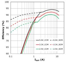
Figure 28: XR76112,  $22V_{IN}$ , 400kHz,  $2.2\mu H$
