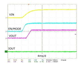
Figure 17: XR76112 Power-up, Forced CCM,  $I_{OUT} = 0A$
