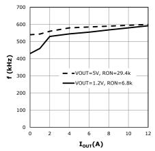
Figure 9: XR76112 Frequency vs.  $I_{\text{OUT}}$ , Forced CCM
