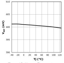
Figure 10:  $V_{\text{REF}}$  vs. Temperature
