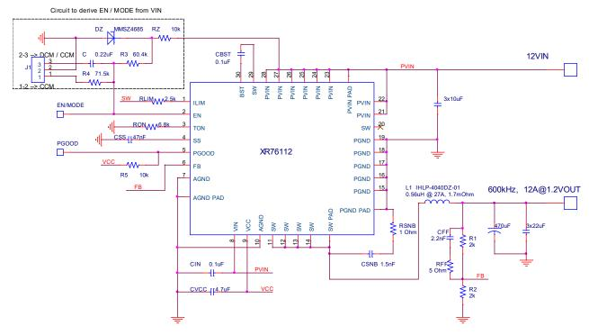
Figure 36: XR76112 Application Circuit Schematic
