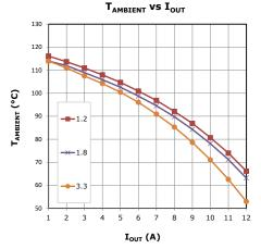
Figure 31: XR76112 Package Thermal Derating,  $12V_{\text{IN}}$
