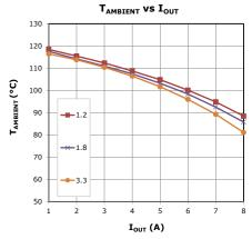
Figure 29: XR76108 Package Thermal Derating, 12VIN
