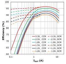
Figure 24: XR76112, 5V<sub>IN</sub>, 600kHz, 0.56µH
