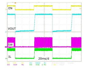
Figure 21: XR76112 Enable Turn On / Turn Off, 1.2Vout, 12A
