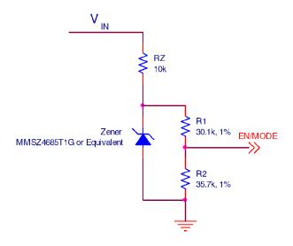
Figure 33: Selecting Forced CCM by Deriving EN/MODE from  $V_{\text{IN}}$
