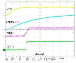
Figure 20: XR76112 Power-up, DCM / CCM,  $I_{OUT} = 12A$
