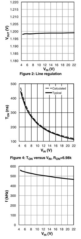
Figure 6: frequency versus V<sub>IN</sub>
