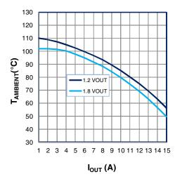
Figure 24: Maximum T<sub>AMBIENT</sub> vs I<sub>OUT</sub>, V<sub>IN</sub>=19.6V
