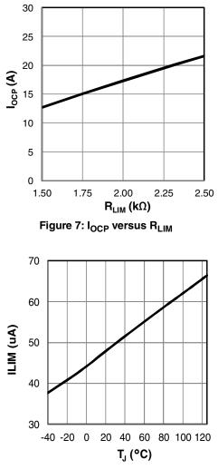
Figure 9: I<sub>LIM</sub> versus temperature
