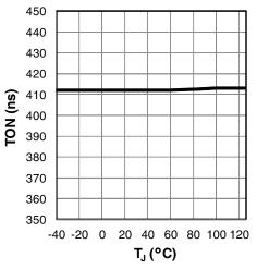
Figure 10: T<sub>ON</sub> versus temperature, R<sub>ON</sub>=16.2k $\Omega$
