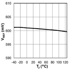
Figure 8: V<sub>REF</sub> versus temperature
