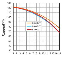
I<sub>OUT</sub> (Α) Figure 20: Maximum T<sub>AMBIENT</sub> vs I<sub>OUT</sub>, V<sub>IN</sub>=5V
