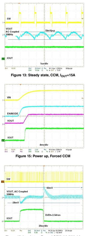
Figure 17: Load step, Forced CCM, 0A-7.5A-0A
