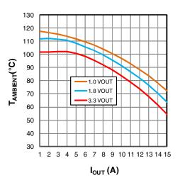
Figure 22: Maximum  $T_{AMBIENT}$  vs  $I_{OUT}, V_{IN}{=}12V$
