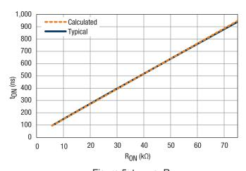
Figure 5.  $t_{ON}$  vs.  $R_{ON}$
