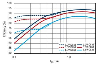
Figure 20. Efficiency,  $V_{IN} = 12V$
