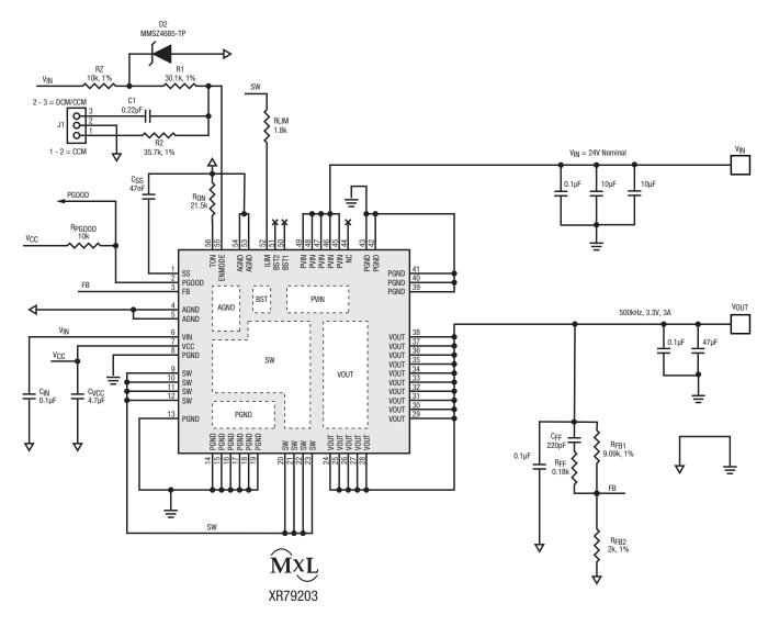
Figure 27. Typical Application Circuit
