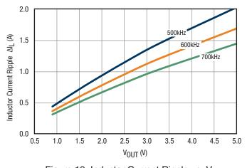
Figure 13. Inductor Current Ripple vs.  $V_{OUT}$
