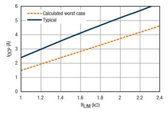
Figure 9. I<sub>OCP</sub> vs. R<sub>LIM</sub>
