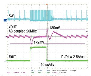
Figure 19. Load Step, DCM/CCM, 0.05A-1.5A-0.05A
