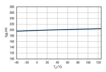
Figure 11.  $t_{ON}$  vs. Temperature,  $R_{ON} = 14k\Omega$
