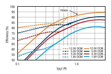
Figure 22. Efficiency,  $V_{IN} = 24V$
