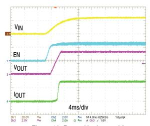
Figure 16. Power Up, I<sub>OUT</sub> = 3A
