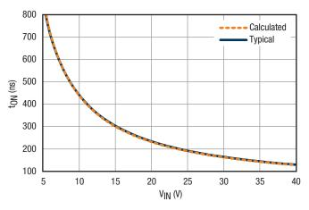
Figure 6.  $t_{ON}$  vs.  $V_{IN}$ ,  $R_{ON} = 14k\Omega$
