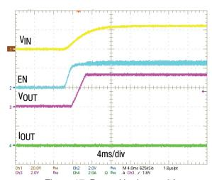
Figure 17. Power Up, I<sub>OUT</sub> = 0A
