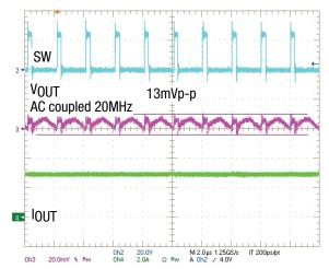
Figure 14. Steady State CCM, I<sub>OUT</sub> = 3A
