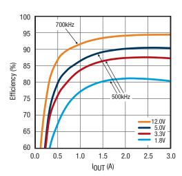
Figure 2. Efficiency, 24V<sub>IN</sub>
