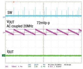
Figure 15. Steady State DCM, I<sub>OUT</sub> = 0A
