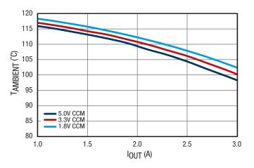
Figure 21. Maximum  $T_{AMBIENT}$  vs.  $I_{OUT}$ ,  $V_{IN} = 12V$
