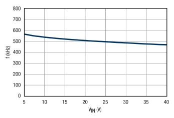
Figure 8. Switching Frequency vs. VIN
