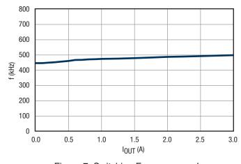
Figure 7. Switching Frequency vs.  $I_{OUT}$
