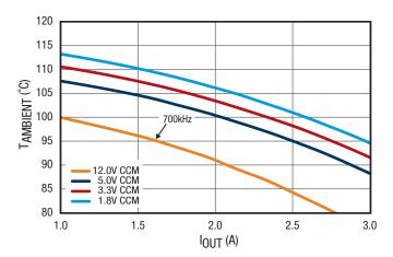
Figure 23. Maximum  $T_{AMBIENT}$  vs.  $I_{OUT}$ ,  $V_{IN} = 24V$
