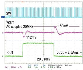
Figure 18. Load Step, CCM, 0A-1.5A-0A
