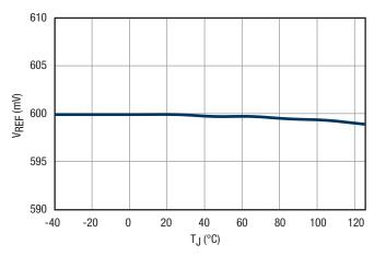
Figure 10.  $V_{\mbox{\scriptsize REF}}$  vs. Temperature
