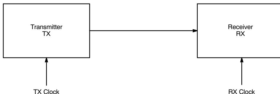
Figure 33. Example of a Serial Data Transmission System
