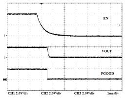
Fig. 17: Shutdown at VOUT = 1.8V
