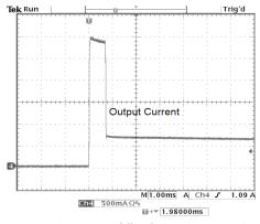
Fig. 20: Current Foldback at VOUT = 1.8V
