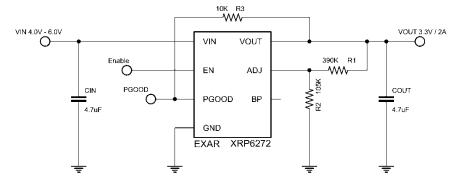
Fig. 23: 5V to 3.3V / 2A
