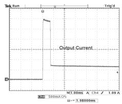
Fig. 21: Current Foldback at VOUT = 3.3V
