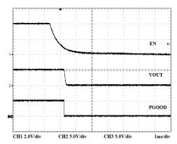
Fig. 19: Shutdown at VOUT = 5V
