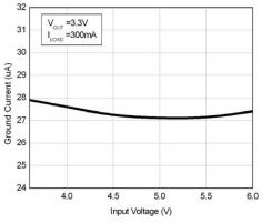
Fig. 7: GND Current vs. VIN at VOUT=3.3V, 300mA
