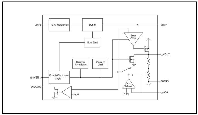
Fig. 2: XRP6272 Block Diagram
