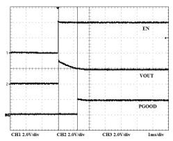
Fig. 16: Enable Startup at VOUT = 1.8V
