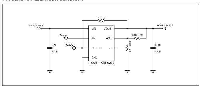
Fig. 1: XRP6272 Application Diagram
