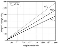
Fig. 12: Dropout Voltage at VOUT = 5.0V
