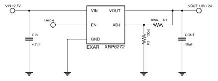
Fig. 25: 2.7V Min to 1.8V / 2A Power Supply
