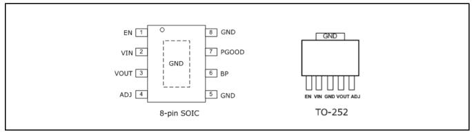
Fig. 3: XRP6272 Pin Assignment
