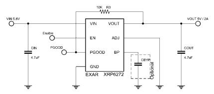
Fig. 24: 5.8V to 5V RF Stage Low Noise Power Supply
