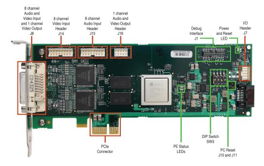
The VRC7008 has a high bandwidth PCIe interface for connectivity with host systems.
