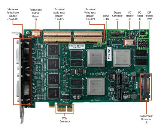
It also supports 16 channels of alarm input-output and an RS485 interface for remote camera control through an I/O header. The card also has a debug connector for UART and JTAG interfaces, which facilitates hardware and software debugging.
