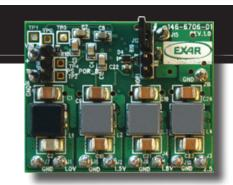
Exar has a slick little quad high-current, programmable, switching power controller IC called the XRP7714 and some recent Googling for "Zynq" uncovered an Exar reference power-supply design that uses the XRP7714 to power a Xilinx Zynq All Programmable SoC. The reference design has a board footprint of 1.875 square inches (1.50 x 1.25 inches) and it looks like (above) on the FET side.
